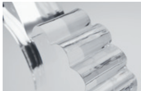
Flame-polished cut of acrylics up to 40 mm
